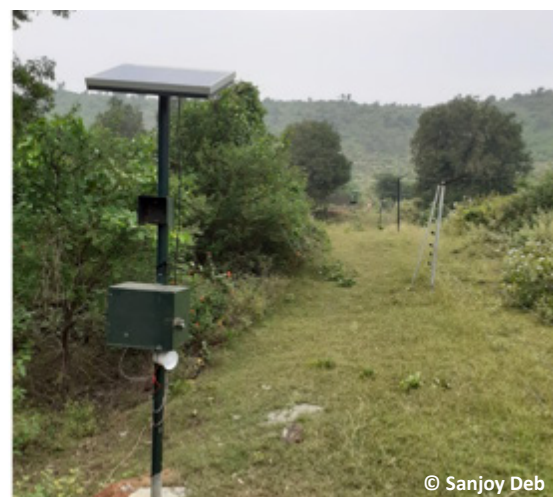
Image 6. A fully functioning Elephant deterrent system unit with hooter.
