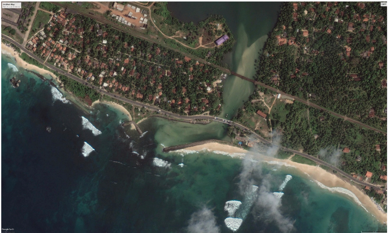
Image 1. Satellite image of lagoon outlet with the existing groyne structures in 2010 (Source: Google Earth Pro 2022).
