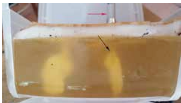
Image 3. Birdseye view of the ballistic gel with mounted pork hide. Depicting the deployed dart (red arrow), and the quality of the drug deposits in the form of clouds within the ballistic gel (black arrow). © D. Rosenfield
