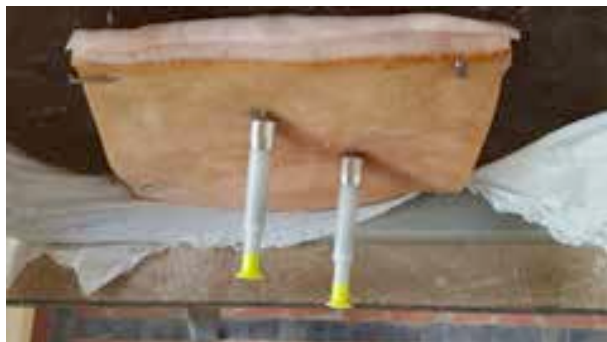
Image 1. Darting – Drug deposit evaluation. Pork hide mounted on a block of ballistic gel with two darts showing full penetration of the dart's cannula. © D. Rosenfield
